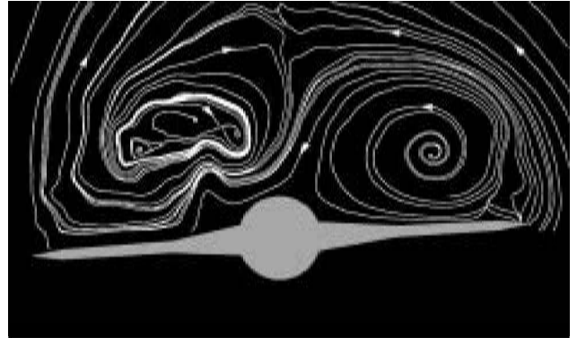
b) Sectional streamline patterns
